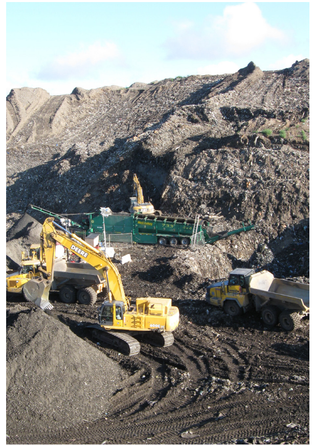
Figure 2 – Waste screening operations – active face in background; stockpiles and processing equipment in foreground.
